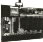
Direct replacement for the A501 Expansion Convenient On/Off RAM Switch ● Autorecharging battery-backed Real-Time Clock Compact unit size
